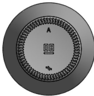
VIEW OF BASE SHOWING EMBOSSED MARKINGS & STANDING AREA EMBOSSED WITH STIPPLES
